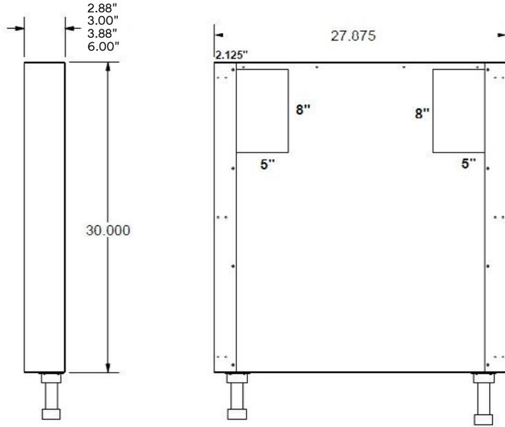
Note: ORP has rectangular cutouts on one side and is finished on front, back, and one side. Reversible for application on either end of a run.
