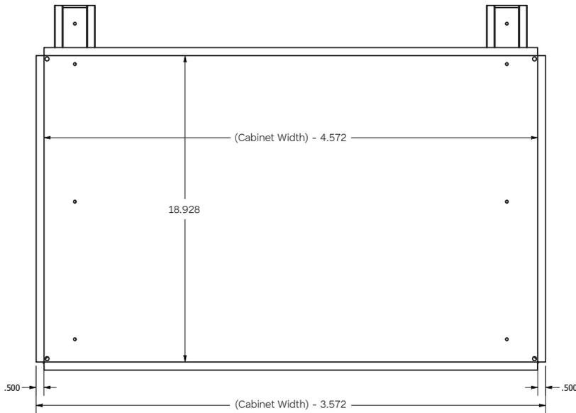
Note: Subtract 3.572" from cabinet width to determine drawer external width. Subtract 4.572" from cabinet width to determine drawer internal width. Drawer depth remains the same regardless of cabinet width.
