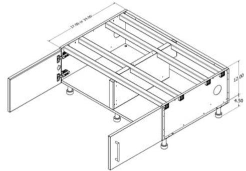
Support bracing beneath top panel shown
