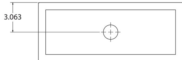
**Note:** Vertical wall cabinet knob placement is the same as base cabinets but handles are placed at the bottom of each door.
