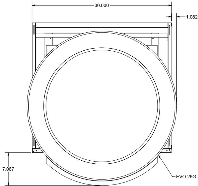
Note: Top view of 25" EVO installed in OGB30xx. There is a 1.08" overhang on the cabinet sides.
