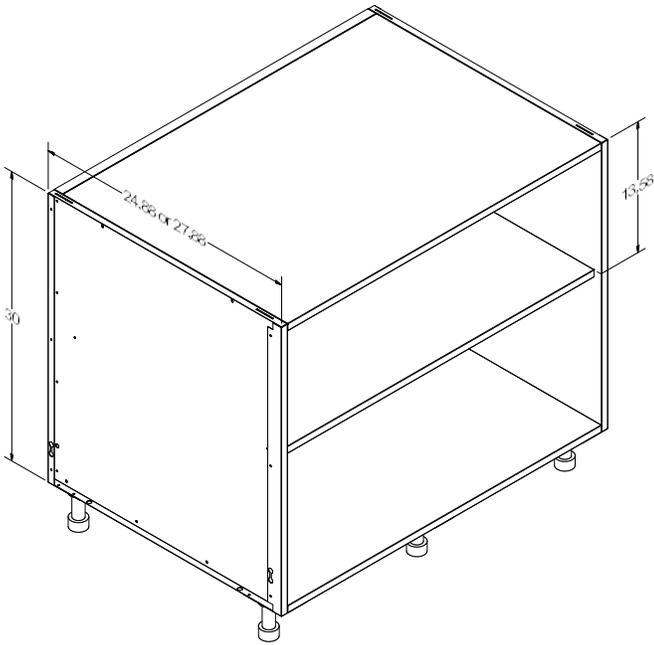
Note: OBFxx00 cabinet box depth is 24.88"D or 27.88"D to match total depth of standard cabinets with fronts. Flush end panels (OFE) are available to finish the exposed side seen when OBFxx00 bases are placed next to standard bases. The return flange on the OBFxx00 side is 7/8" longer to line up with adjacent sides.
