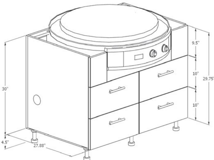
Note: 25" and 30" EVO grills installed in 33" wide base will overhang the cabinet sides and back slightly. Please see following page for top view and additional specifications.
