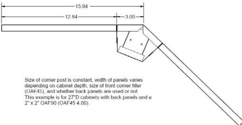
Size of corner post is constant, width of panels varies depending on cabinet depth, size of front corner filler (OAF45), and whether back panels are used or not. This example is for 27"D cabinets with back panels and a 2" x 2" OAF90 (OAF45 4.00).
