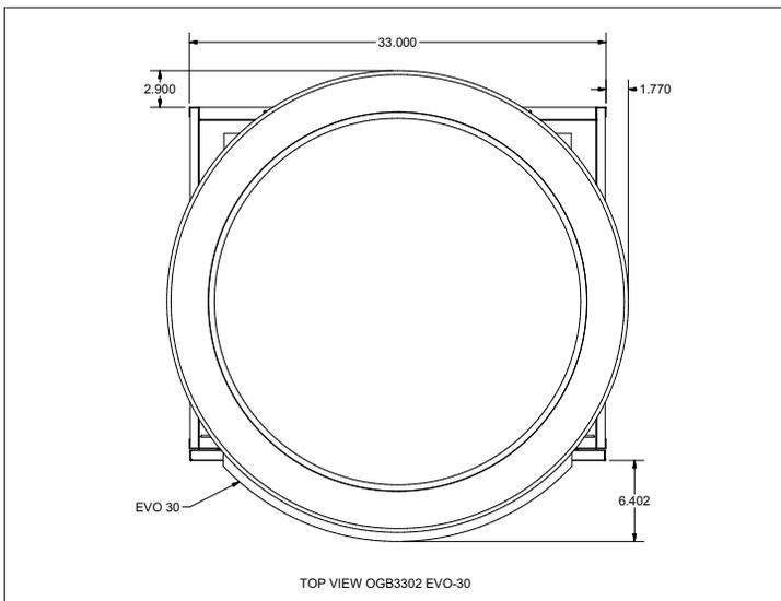
**Note:** Top view of 30" EVO installed in OGB3302. The grill overhangs 1.77" on the side as well as 2.9" on the cabinet back.
