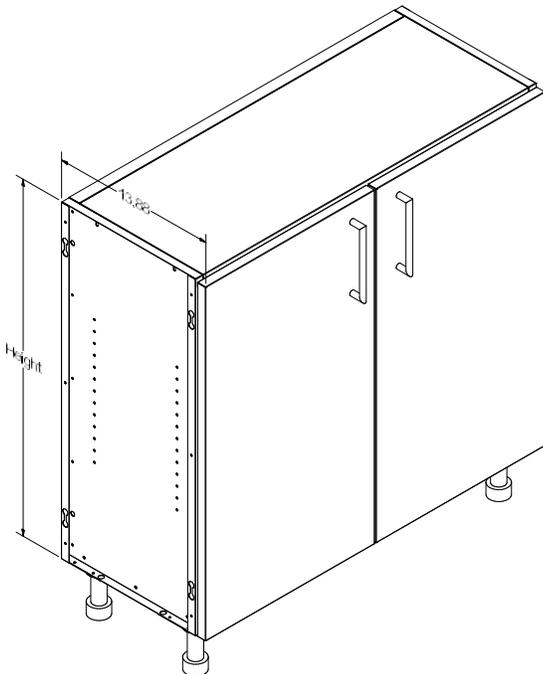
NOTE: Cabinets may tip if not attached to 24" or 30" depth cabinets. Please observe all local building codes when installing. Cabinet boxes are 30" or 36" high plus 4.5" leveling legs or 2" (ADA) leg heights. Decorative side panels are available in every door style.
