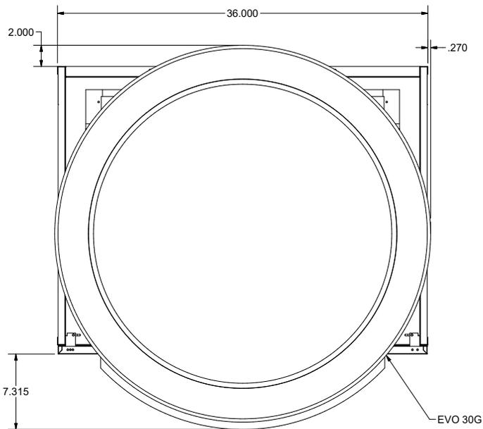
Note: Top view of 30" EVO installed in OGB36xx. The grill overhangs .27" on the sides as well as 2" in the back.
