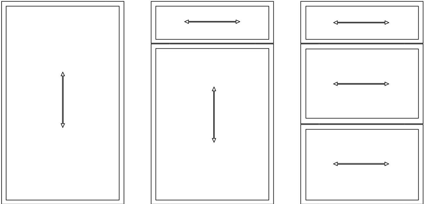
**Note:** Venice doors can ONLY have the center panel wood grain powder coated and the frame left as stainless steel or powder coated a standard color. Wood grain centers are coated with standard vertical orientation shown above.
