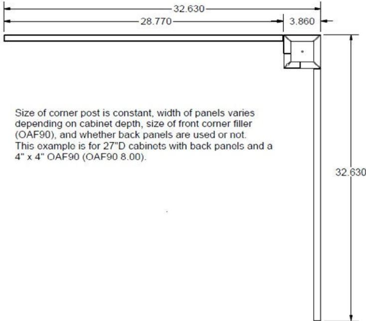
Size of corner post is constant, width of panels varies depending on cabinet depth, size of front corner filler (OAF90), and whether back panels are used or not. This example is for 27"D cabinets with back panels and a 4" x 4" OAF90 (OAF90 8.00).
