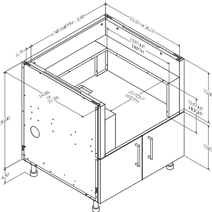
Note: Inner trim dimensions of OBBxx02 LOW adjust based on the power burner selected. Power burner cutout must be at least 7.5" LESS than cabinet size selected due to trim kit requirements.
