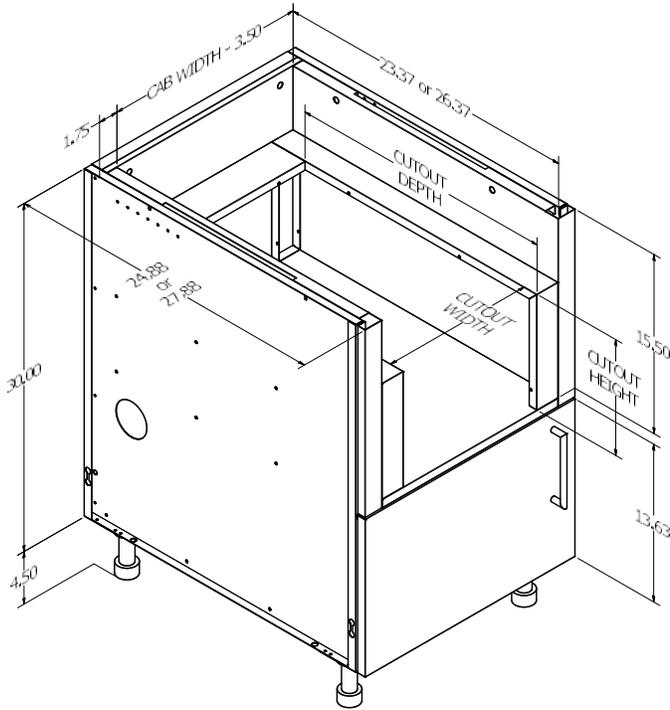
Note: Inner trim dimensions of OBBxx01 LOW adjust based on the power burner selected. Power burner cutout must be at least 7.5" LESS than cabinet size selected due to trim kit requirements.
