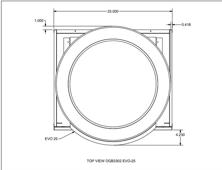
**Note:** Top view of 25" EVO installed in OGB3302. There is no overhang on the cabinet sides but it does overhang by 1" on the cabinet back.
