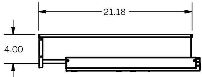
Note: Subtract 3.97" from cabinet width to determine drawer external width. Subtract 4.22" from cabinet width to determine drawer internal width. Drawer depth remains the same regardless of cabinet width.
