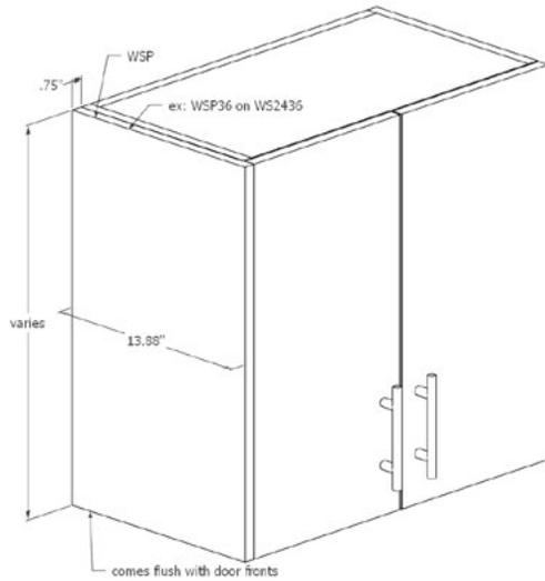
**Note:** Decorative side panels to match door fronts can be applied using Part: **WSP DECORATIVE L/R** and filling in the height (ranging from 15"-42" in 3" increments), depth (13.88" or 24.88"), side (left or right), and door style.
