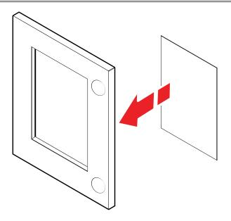
4. The glass will sit on the preinstalled gaskets inside the door rear panel and should sit approximately as shown.
